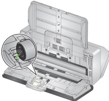
5. Re-install the pre-separation pad (or install a new one) by aligning the slots with the holes on the pre-separation pad and snapping it into place.
