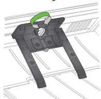
2. Hold the stacking deflector slightly in front of and lower than the front lower edge of the scanner cover, with the legs pointing away from the scanner.
