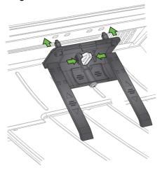
5. Turn the locking knob horizontal into its locked position. The stacking deflector is now held in place on the scanner. When the deflector is
