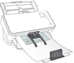
4. If scanning pages of several different lengths (for example 3 inches, 5 inches, and 11 inches long), adjust the deflector legs so they will trap all the shorter pages. In this example, adjust to trap the 5 inch pages. The shorter pages will stay near the scanner, and the longer pages will push beyond the stacking deflector legs.
