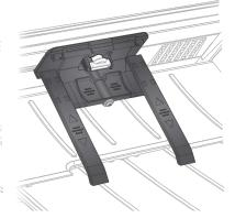
installed correctly, they will touch the partially extended output tray.
