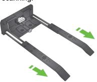
3. When scanning pages of different lengths (such as a form accompanied by a check), adjust the stacking deflector accessory legs so they will trap the shorter page. The longer pages will push under the deflector legs, but shorter pages will stay close to the scanner.
