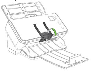
Flip the stacking deflector down again when needed. The stacking deflector is *not* recommended for lightweight pages longer than 150 mm (5.9 inches).
