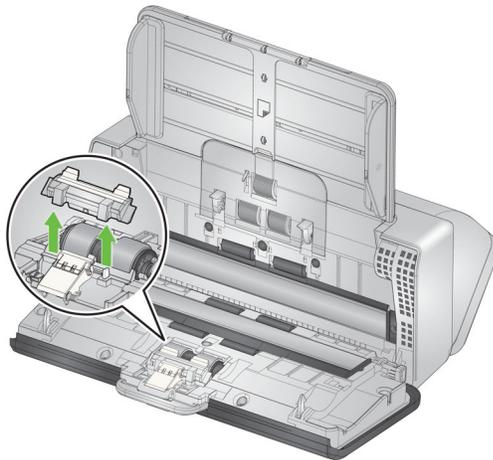
3. Grasp the separation roller and pull it straight out.
