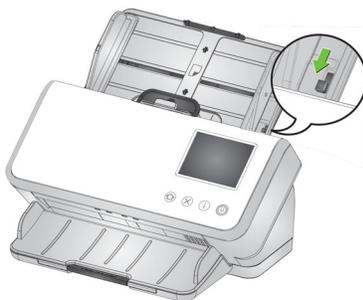
7. Extend the output tray so it is longer than the input stack by about 1/2 in/1 cm. Raise the end stop of the output tray, if the paper is shorter than 14 in/35 cm.
