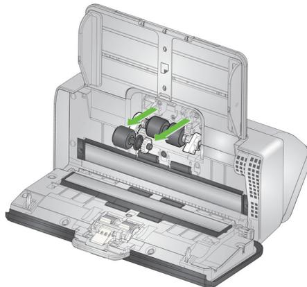
4. Reinstall the urging roller, aligning it correctly.
