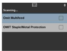
3. After scanning documents that require you to use the Omit option, select **Toggle** which allows you to enable or disable the misfeed detection and metal protection features for any number of documents.
