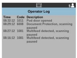
The messages that are displayed in the log are only those messages that have occurred since the scanner was powered on. When you turn the power off or the scanner goes into Standby or Low Power mode, the Operator Log on the Operator Control Panel will be cleared.
