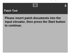
Place a document(s) with a patch(es) in the input elevator and press the Start/Pause button. When the documents have been scanned, the results of the patch test will be displayed. The results show the number of toggle patches that were recognized by the scanner.
