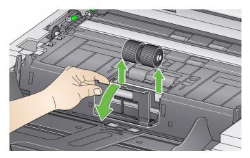
6. Manually rotate and wipe the separation roller tires with a roller cleaning pad. For best results wipe parallel to the ribs in order to remove any residue between the ribs.
