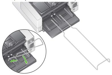
Adjusting the output tray for rear edge alignment or improved or best document handling
