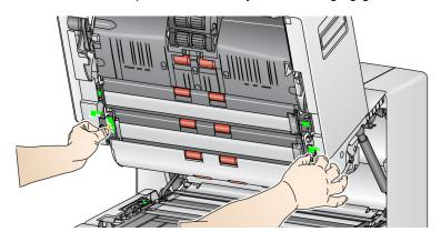
4. Carefully vacuum the area between the LEDs.
