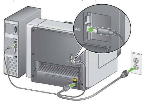
6. Secure the USB cable into the cable routing channel on the back of the scanner.
