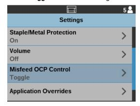
Select One Page to access the Omit options for the multifeed and metal protection feature which allows you to disable the feature for single documents. Recheck Omit as needed for other documents in the same scan job.
