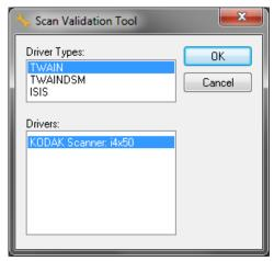
4. Select **TWAIN** for the Driver Type and the **KODAK Scanner: i4x50**. The Scan Validation Tool dialog box will be displayed.
