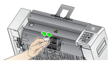
10. Inspect the tires. If the tires show signs of wear or damage, replace the feed module tires. See "Replacement procedures" later in this chapter.
