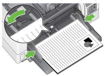
Adjusting the height of the input elevator — the input elevator can be set to accommodate stacks of 25-, 100-, 250- or 500-documents of 20 lb. /80 g/m<sup>2</sup> bond paper. Input elevator settings are typically made through your scanning application software (e.g., TWAIN Datasource or ISIS Driver).
