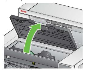
NOTE: If you do not want to remove the output tray, you can lift the front of the output tray, then lift the printer access cover and position the printer access cover behind the height adjustment tab.
