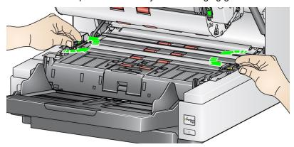
9. Carefully vacuum the area between the LEDs.
