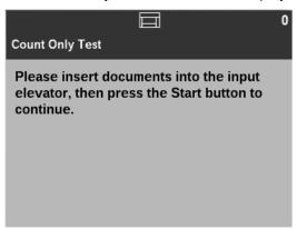
Place the documents you want to count in the input elevator and press the Start/Pause button. When the scanner has fed all documents, the total number will be displayed in the Status area.
