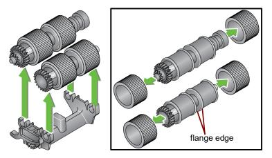
Install each new tire by gently pulling it over the core. The tires do not need
