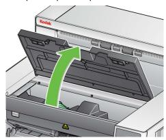
NOTE: If you do not want to remove the output tray, you can lift the front of the output tray, then lift the printer access cover and position the printer access cover behind the height adjustment tab.
