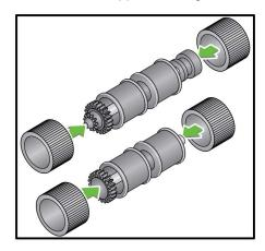
Replacing the feed module
