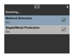
2. Choose **One Page** to access the Omit options for the multifeed and metal protection features which allows you to disable the feature for single documents. Recheck **Omit** as needed for other documents in the same scan job.
