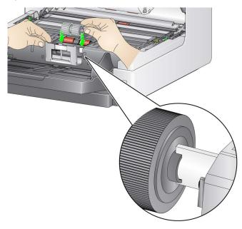
5. Gently lower the roller cover back in place and close the scanner cover.
