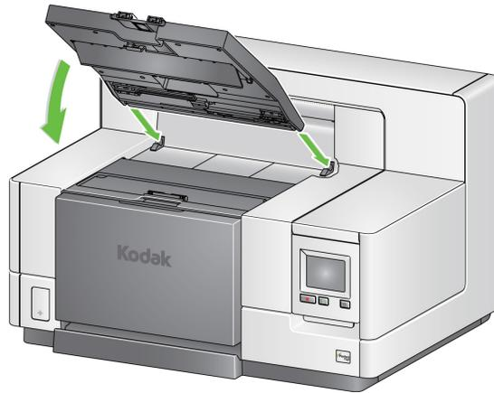
**NOTE:** Be sure to lift the output tray up to the scanning position before feeding documents. See “Adjusting the output tray” on page 19.
