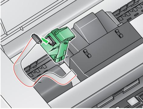
**NOTE:** If you are replacing an ink cartridge, the printer cable will already be installed and you just need to remove the printer carrier from its position and remove the empty ink cartridge.
