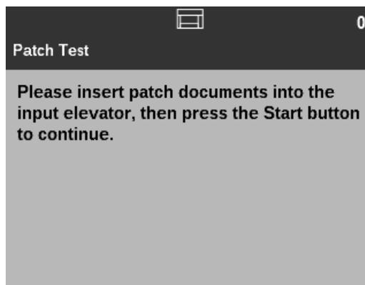
2. Place a document(s) with a patch(es) in the input elevator and press the **Start/Pause** button. When the documents have been scanned, the results of the patch test will be displayed. The results show the number of toggle patches that were recognized by the scanner.
