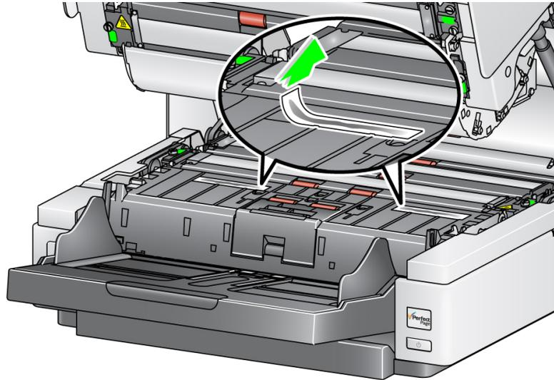
5. Remove the backing from a new blotter strip.
