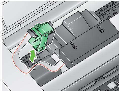
4. Open the ink cartridge package and remove the tab from the new ink cartridge.
