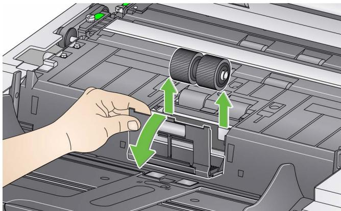
6. Manually rotate and wipe the separation roller tires with a roller cleaning pad. For best results wipe parallel to the ribs in order to remove any residue between the ribs.
