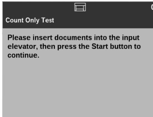
2. Place the documents you want to count in the input elevator and press the **Start/Pause** button. When the scanner has fed all documents, the total number will be displayed in the Status area.
