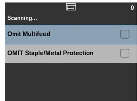
3. After scanning documents that require you to use the Omit option, select **Toggle** which allows you to enable or disable the misfeed detection and metal protection features for any number of documents.
