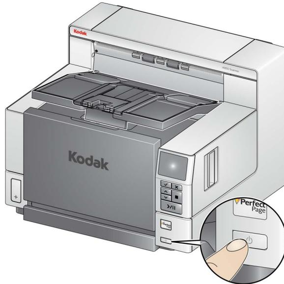
When you turn on the scanner, the input elevator will open if it is not already opened and the green indicator on the **Start/Pause** button will flash as the scanner goes through a series of self tests.
