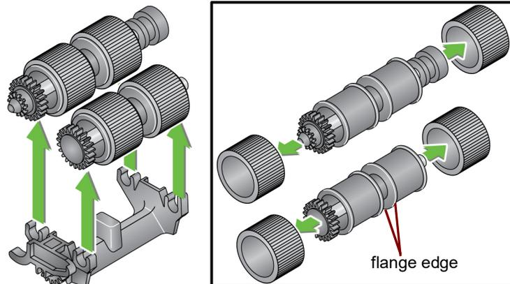
9. Install each new tire by gently pulling it over the core. The tires do not need to be installed in any specific orientation. Make sure that the tires are fully aligned with the flange edge. If they are improperly aligned, premature wear of the tires may occur.
