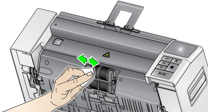
10. Inspect the tires. If the tires show signs of wear or damage, replace the feed module tires. See “Replacement procedures” later in this chapter.
