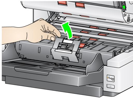
**NOTE:** The separation roller cover is spring-loaded. Hold the separation roller cover back until you remove the separation roller, then gently lower the roller cover back in place.
