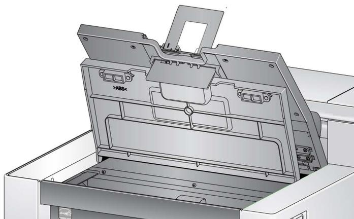
4. Turn the feed module release knob and release the feed module.
