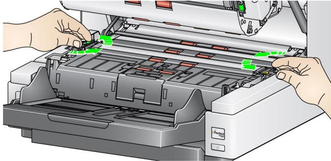
4. Install the new imaging guide and tighten the screws to secure the imaging guide.
