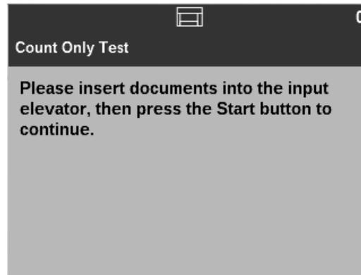
2. Place the documents you want to count in the input elevator. As the scanner is counting documents, when a multifeed is encountered, the scanner will stop.
