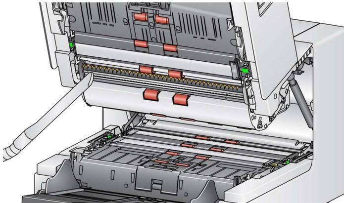
5. Clean both the top and bottom of the imaging guide thoroughly with a Staticide wipe or a “Step 1” Brillianize Detailer wipe.
