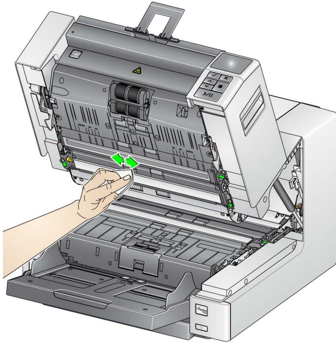
4. Wipe the upper and lower imaging guides again with an almost-dry Staticide wipe or a “Step 2” Brillianize Detailer wipe to remove any streaks.
