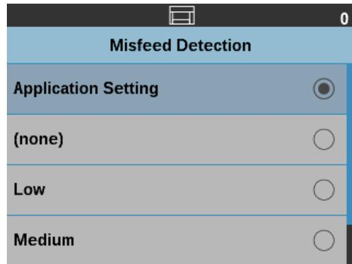
3. Select one of the misfeed detection options. When **Low**, **Medium** or **High** is selected, multifeed detection will be enabled with the Interactive Multifeed action and all three sensors will be turned on. The Intelligent Document Protection feature will also be enabled.
