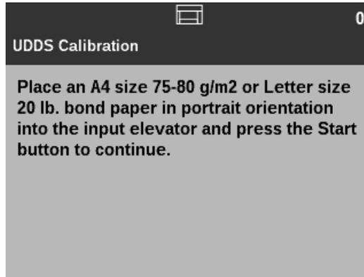
2. You will be prompted to place an A4 size 75-80 g/m<sup>2</sup> or lettersize 20 lb. bond sheet of paper in the input elevator in portrait orientation.
