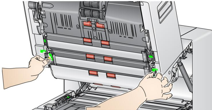
4. Carefully vacuum the area between the LEDs.
