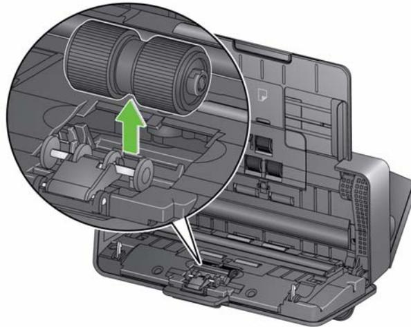
3. Wipe the separation roller tires with a roller cleaning pad.
