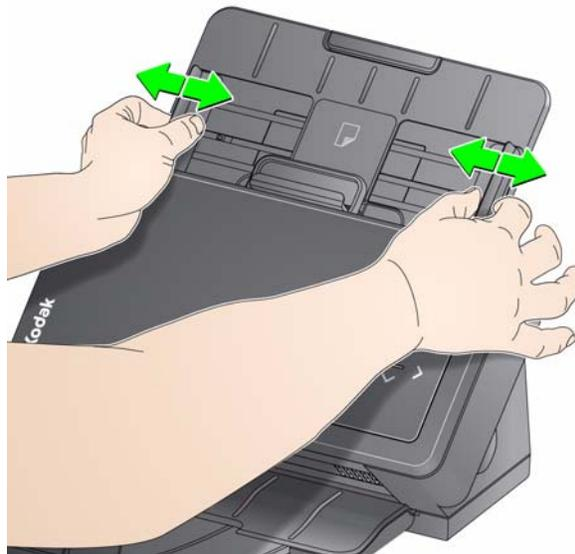
3. If necessary, adjust the input and output trays to accommodate your scanning needs. The output tray can be extended to accommodate documents up to 35.56 cm (14 inches) in length. An end stop is available to accommodate document stacking. Lift this end stop as needed for scanning documents up to A4 (11.7 inches).
