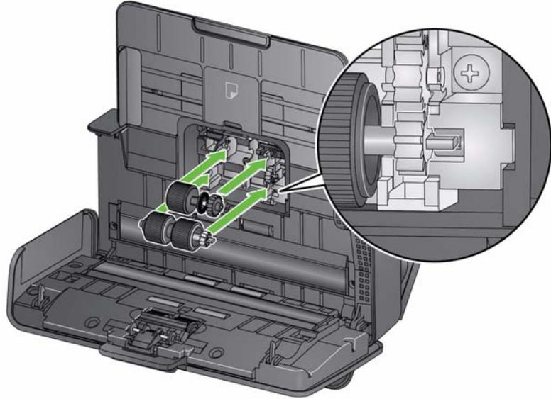
8. Reinstall the top feed roller.
