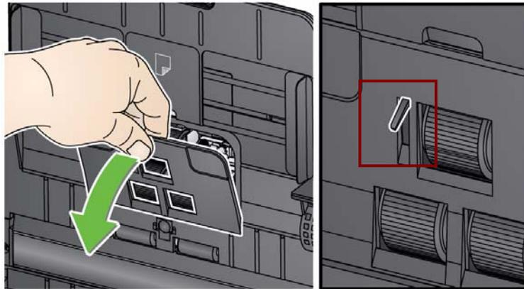
**NOTE:** Be careful not to damage the paper present sensor when removing or cleaning around the feed roller.
