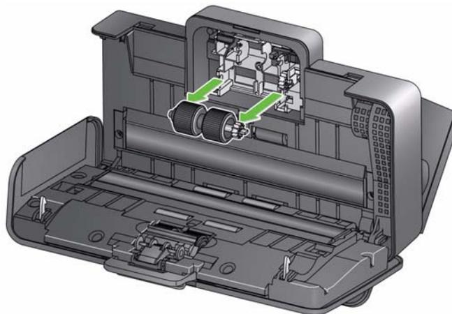
3. Rotate the lower feed roller so the pin is positioned with the open slot, then lift the roller out of position.
