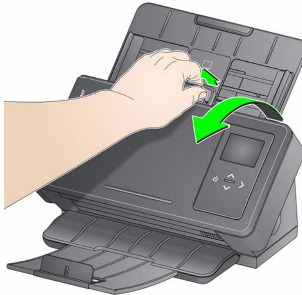
2. When you finish cleaning the scanner or replacing a part, close the scanner cover.
