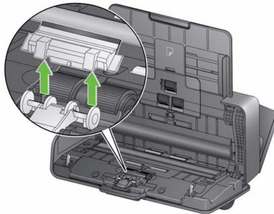
2. Remove the separation roller.
