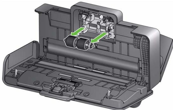
4. Rotate the lower feed roller so the pin is positioned with the open slot,
