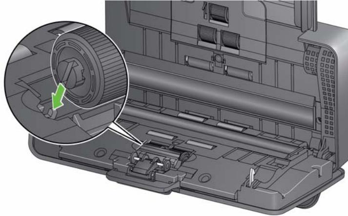
6. Re-install the pre-separation pad by aligning the slots with the holes on the pre-separation pad and snapping it into place.
