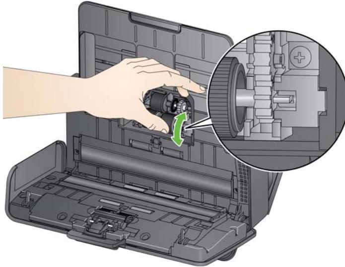
then lift the roller out of position.
