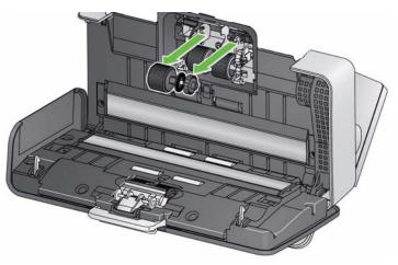
4. Rotate the lower feed roller so the pin is positioned with the open slot.
