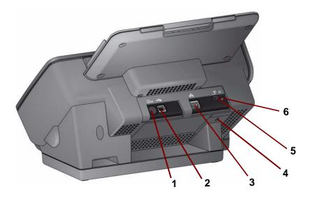
1 24V ---- Power port — connects the power supply to the scanner.
