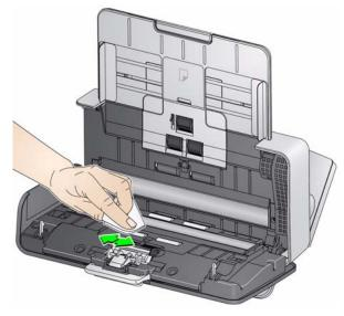
IMPORTANT: The roller cleaning pad contains sodium lauryl ether sulfate which can cause eye irritation. Refer to the Safety Data Sheet (SDS) for more information.
