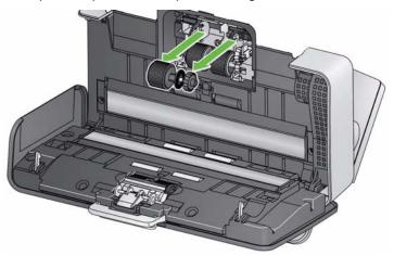
3. Rotate the lower feed roller so the pin is positioned with the open slot, then grasp the lower feed roller and pull it straight out.
