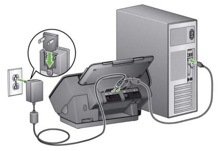
NOTE: Do not plug in an Ethernet cable and a USB cable at the same time into the back of the scanner; the scanner will not function in this configuration. The Device tab provides the following options.
