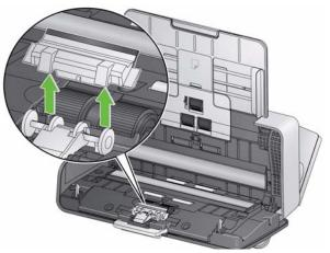
2. Grasp the separation roller and pull it straight out.
