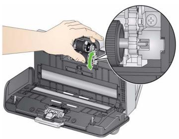
then grasp the lower feed roller and pull it straight out.
