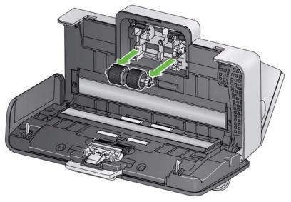
4. Install a new lower feed roller and top feed roller by aligning the pins with the open slots and fitting each roller into position. Be sure the gears are aligned and the roller snaps into place.
