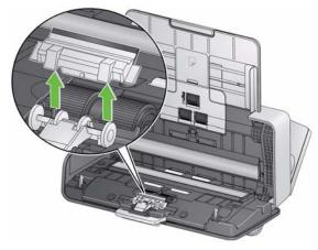
2. Remove the separation roller.
