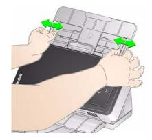
3. If necessary, adjust the input and output trays to accommodate your scanning needs. The output tray can be extended to accommodate documents up to 35.56 cm (14 inches) in length. An end stop is available to accommodate document stacking. Lift this end stop as needed for scanning documents up to A4 (11.7 inches).
