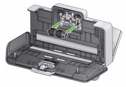
5. Wipe the top and lower feed roller tires with a roller cleaning pad.
