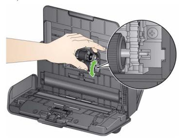
then lift the roller out of position.
