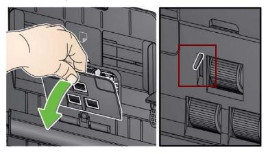
NOTE: Be careful not to damage the paper present sensor when removing or cleaning around the feed roller.
