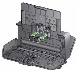
4. Install a new lower feed roller and top feed roller by aligning the pins with the open slots and fitting each roller into position. Be sure the gears are aligned and the roller snaps into place.
