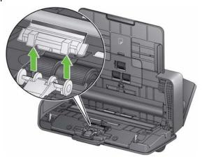
2. Remove the separation roller.
