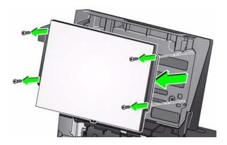
3. Align the new flatbed and insert and tighten the screws until the flatbed background is secure.
