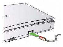
3. Attach the other end of the cable to the scanner.
